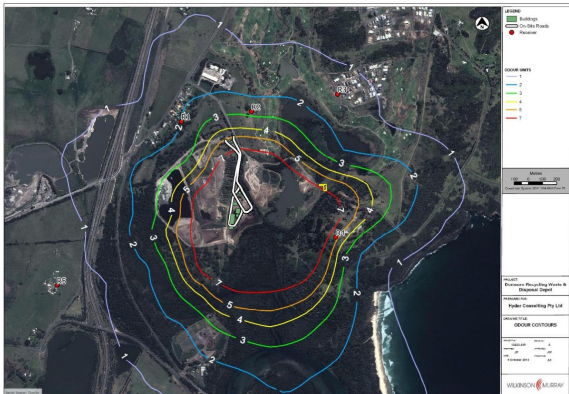
Figure 12: An 'odour contour' map from the Odour Assessment, indicating the odour unit modelling (1 = least offensive, 7 = highest tolerance for residential properties).
